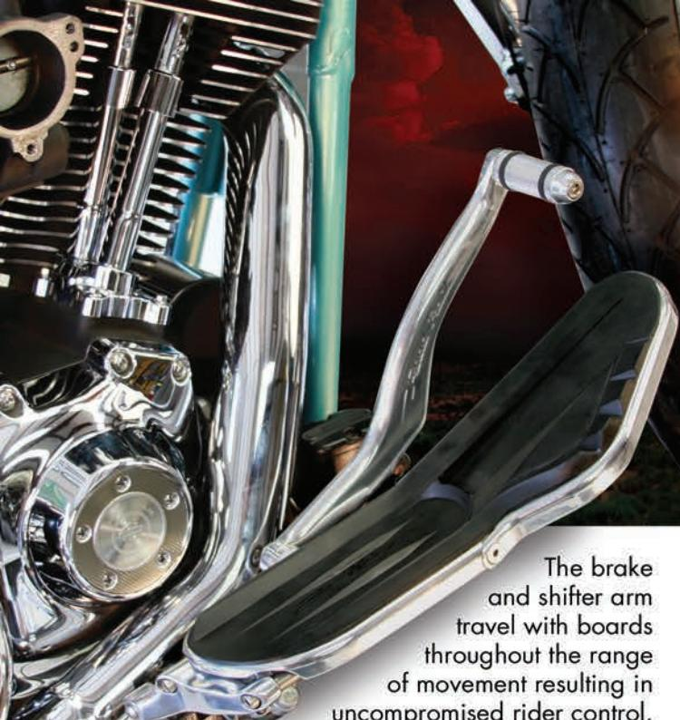
The brake and shifter arm travel with boards throughout the range of movement resulting in uncompromised rider control.
